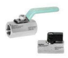
Optional sour gas service conforms to NACE Mr0175. Ball valves are hydrostatic tested at the full rated pressure and low pressure pneumatic at 70 psi. 100% factory test.
