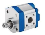
This efficiency is achieved through pressure-based gap sealing and high-precision manufacturing technology. Rexroth external gear pumps are available in four platforms: B, F, N and G, with different gear widths within a platform for different displacements. The pumps come in Standard, High-Performance, SILENCE and SILENCE PLUS versions. Different flanges, shafts, valve arrangements and multiple pump combinations produce additional variants for each version.
