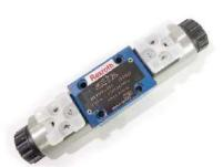
Direct operated directional spool valve with solenoid actuation in heavy-duty design, Subplates, see data sheet RE 45054 (separate order). Wet-pin DC or AC solenoids with detachable coil. Solenoid coil can be rotated 90°. The pressure-tight chamber needs not to be opened for changing the coil. Electrical connection as individual or central connection, Manual override, optional. Inductive position switches and proximity sensors.
