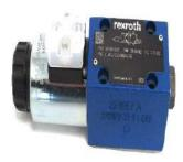
Direct operated directional spool valve with solenoid actuation in high-performance design. Porting pattern according to DIN 24340 form A. Porting pattern according to ISO 4401-03-02-05 and NFPA T3.5.1 R2-2002 D03. Subplates see data sheet RE 45052. Wet-pin DC or AC voltage solenoids with detachable coil. Solenoid coil can be rotated by 90°. The coil can be changed without having to open the pressure-tight chamber. Electrical connection as individual or central connection and manual override.
