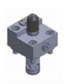
Model CV in cavities machined as per ISO 7368, and provide facility to use the cartridge valve as a leakage free pilot operated check valve, when its pilot port Z1 is connected to port B of the cartridge. In this condition, the combination allow free flow from its port A to port B and free reverse flow from port B to port A when its pilot port X is pressurised.
