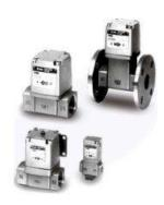
The VND series is a 2-port valve for steam control up to 180°C. It is available with copper alloy or stainless-steel body and also as normally open or normally closed valve. Process valve series VND, Air operated type, Orifice size: 7 to 50mm, Port size: 1/8-to-2-inch, Operating pressure range: 0 to 0.97 MPa
