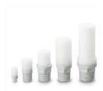
AN05 to 40, Silencer, Compact Resin, Male Thread. Series AN silencers offer various styles and low back pressure in a compact, easy mounting design. The noise reduction has been improved to 30 dB(A) and the case is UL94-V0 grade, flame resistant material. Series AN is available with M, R or NPT threads. RoHS Compliant. More compact: 30% length reduction, 25% outside diameter. Improved noise reduction: 30dB(A). Connection method: M, R, NPT threads.
