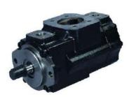
These double pumps consist of two HPV2 series single pumps combined in tandem within a single housing and driven by a common shaft. Fluid delivered from the two-separate ports can be either supplied to separate or common circuits. These HPV pumps are designed for high-pressure functions. Suitable for mobile applications like Drill rigs, Railways & Construction Equipment.
